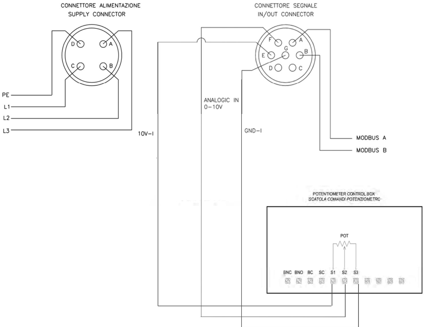
**NB: It is necessary pull the A and B wires down to the control box for the Modbus connection, used for maintenance and diagnostic actions.**
