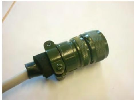
*USE AROUND CABLE ONE SHEATH TO INCREASE THICKNESS AND HAVE OPTIMUM CLOSING*
