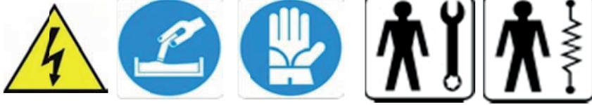
**Before doing any maintenance work, isolate the equipment from the power supply!**
