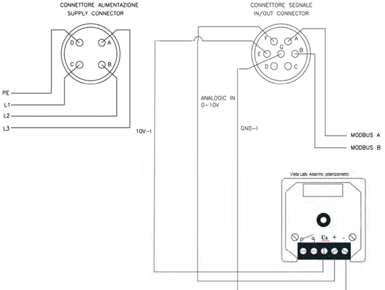
**NB: It is necessary pull the A and B wires down to the control box for the Modbus connection, used for maintenance and diagnostic actions.**
