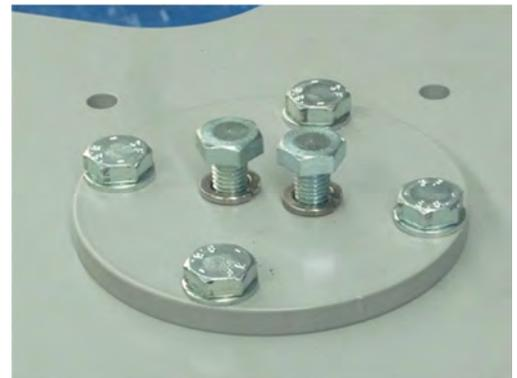
*PLACE BLADE SUPPORT WITH DISC OVER THE SHAFT AND CLAMP SCREWS M10x35 TE WITH NUTS GROWER D.10*
